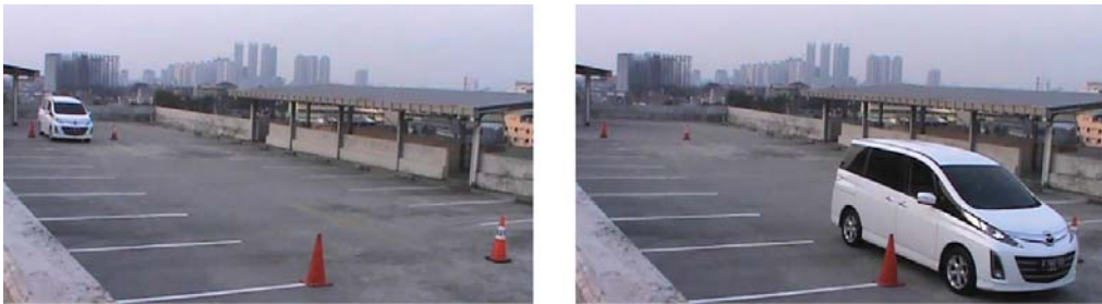
Fig. 3. The test vehicle initial and final positions and the four cones used for orthorectification.
